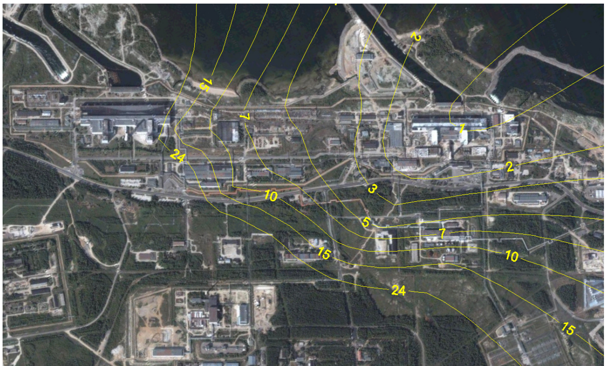
Fig. 3. Time isoline (h) of the personnel staying on the industrial site under condition of 1 mSv daily dose non-exceeding.
